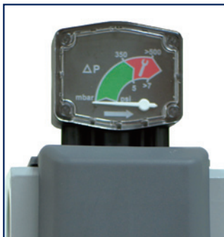
Differential Pressure Gauge
